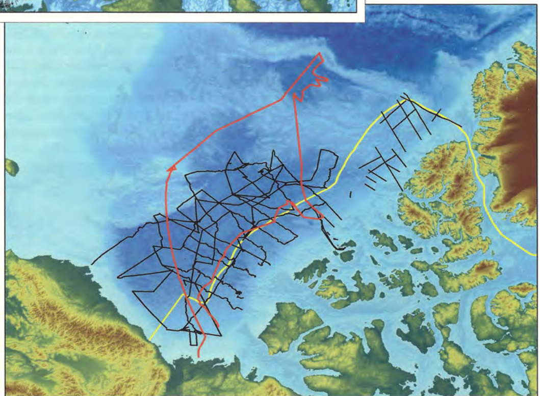
Figure 8 : Seismic coverage in the Western Arctic including the fall joint survey in 2011 (red line)
