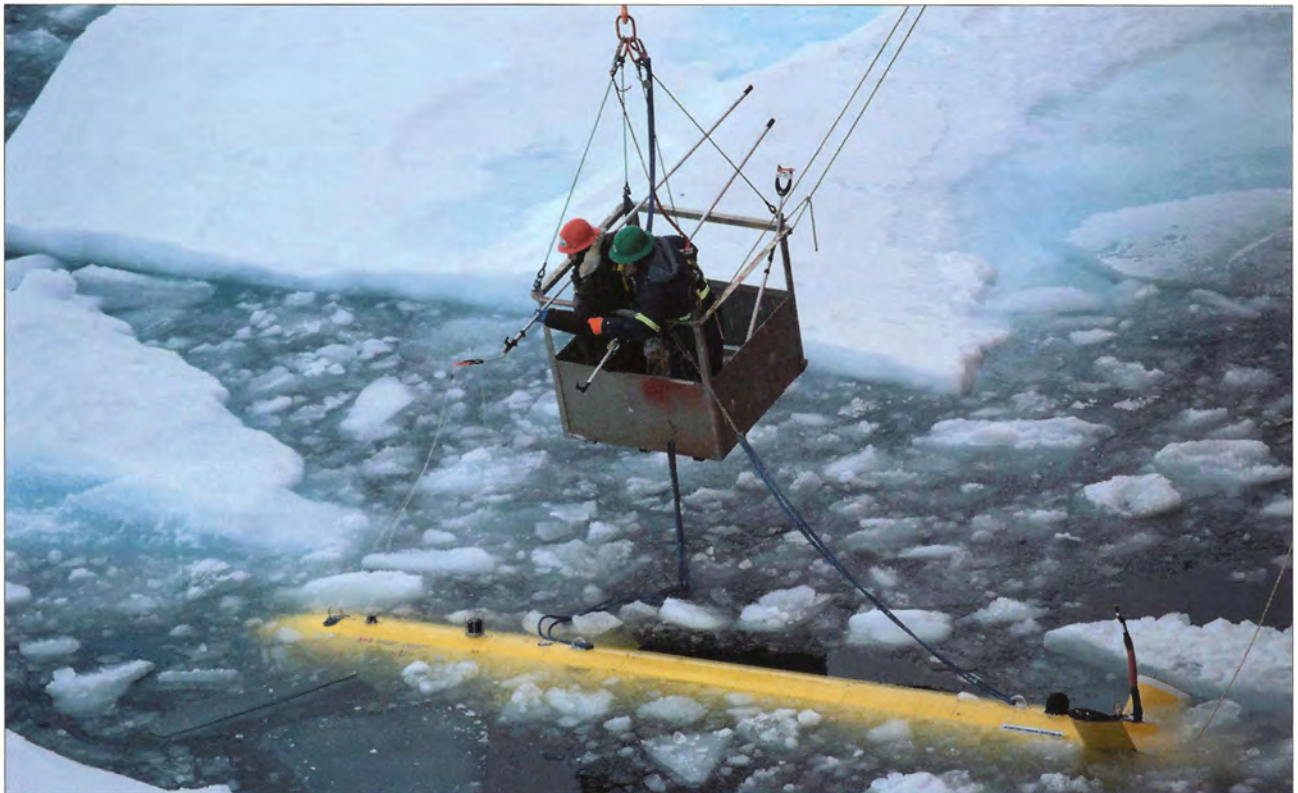
Figure 10 : Recovering the AUV in Arctic waters
