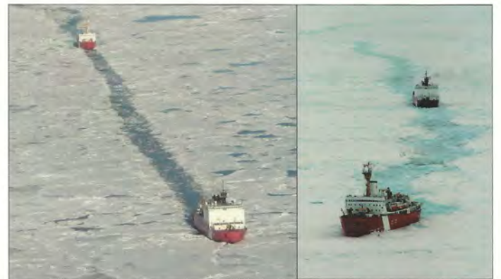
Figure 6 : On left USCGC Healy leading (seismic data priority); on right CCGS Louis S. St-Laurent leading (multi-beam bathymetry priority)
