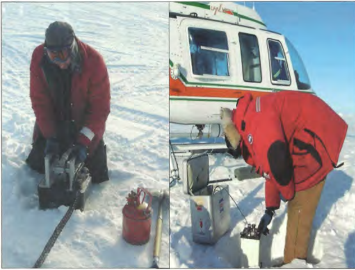
Figure 4 : Collecting bathymetry and gravity to determine the shape of the seafloor
