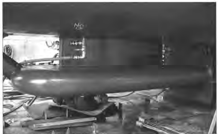
Figure 12: BMT gondola design 2, as modified by Allied shipyard with additional CCG input.
