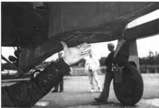
Figure 2: Puffin in-keel fairing of EM3000.
