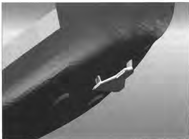
Figure 11: Mantech gondola design (modified) shown on Vector hull with existing sonar blisters.
