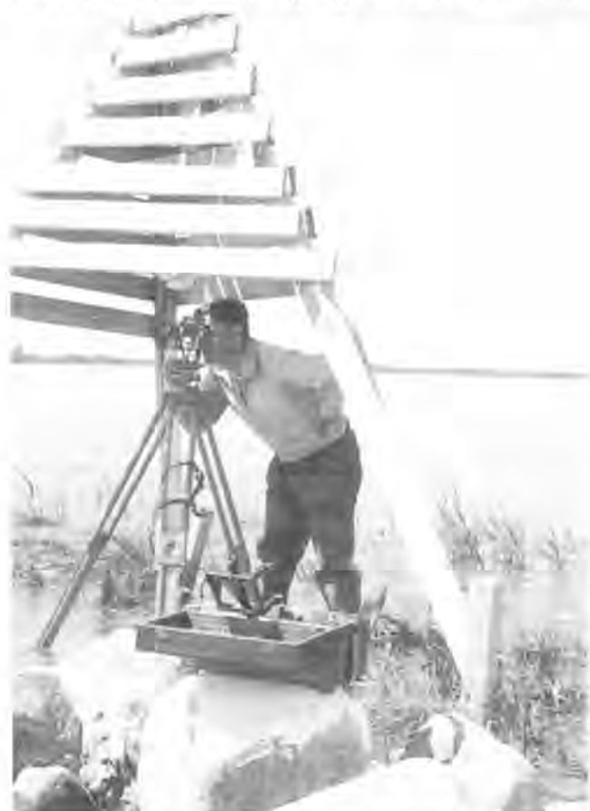
Sid van Dyck observing angles at a main triangulation station.
