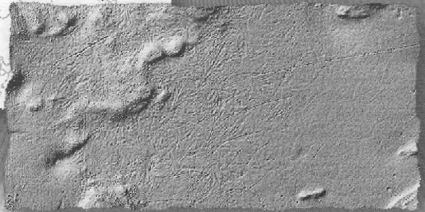
Shaded depth presentation to reveal more details on seafloor (possibly anchor tracks shown above) - EM 3000 built in software.
