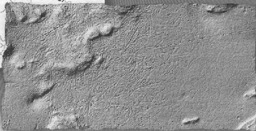
Shaded depth presentation to reveal more details on seafloor (possibly anchor tracks shown above) - EM 3000 built in software.
