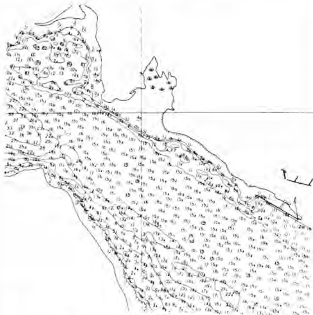
Figure 3: Chart Data with Overplot Removed. Shoals with 50% Margins and Deeps with 2000 % Margins
