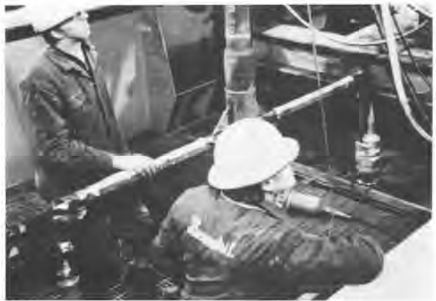
FIGURE 12 DEPLOYMENT OF SONAR 971 AND SONARDYNE ACOUSTIC POSITIONING TRANSDUCER ON MOLIKPAQ DRILLPIPE
