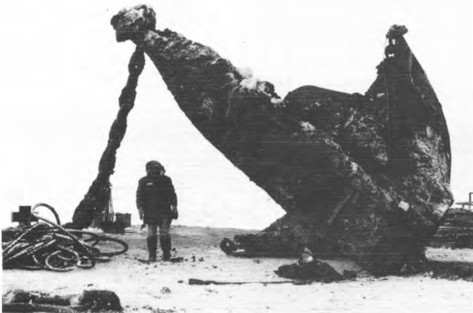
FIGURE 7 AUTHOR WITH A RECOVERED 15 TON BRUCE ANCHOR
