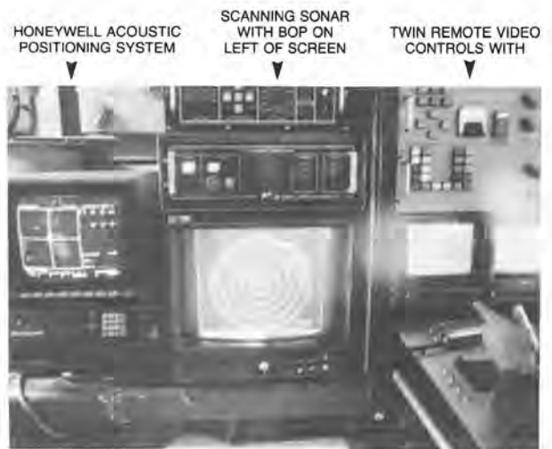
FIGURE 9 BOP DISPLAYED ON VIDEO WITH SONAR IN IMAGING MODE
