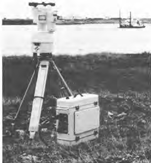
Fig. 1: POLARFIX laser positioning of dredger.
