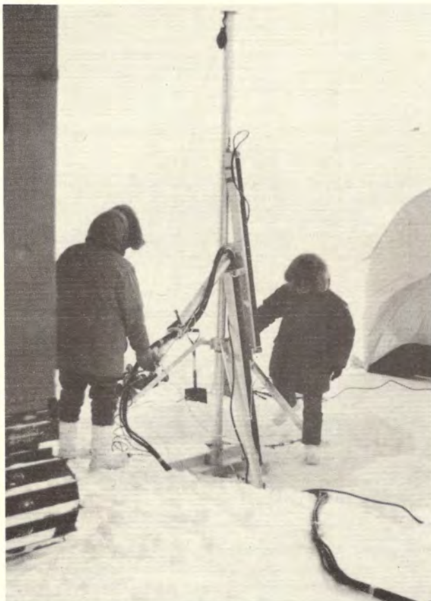
Figure 20: Transducer Assembly Being Lowered Through the Ice
