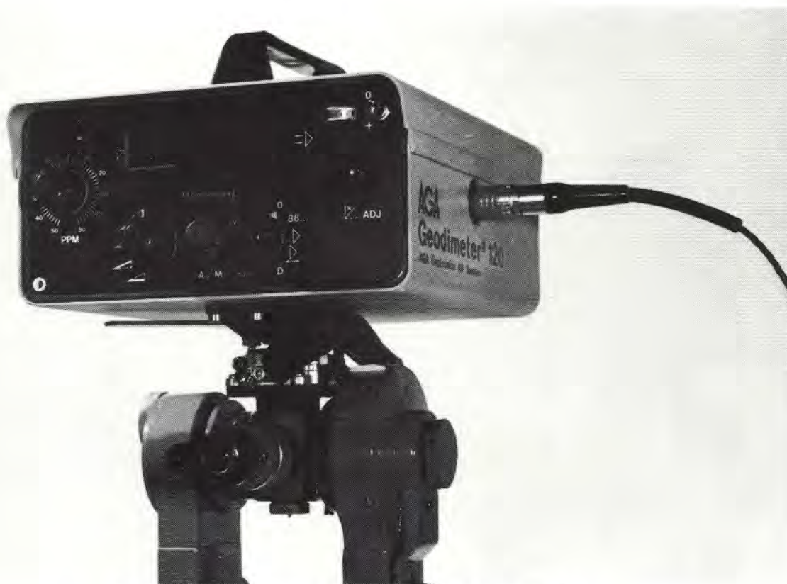
Figure 1: AGA Geodimeter 120 mounted on Wild T-2 Theodolite.
