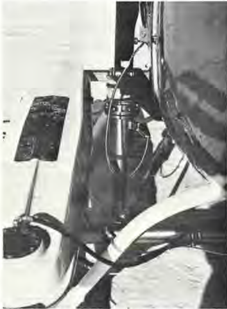
Electrically Actuated Spike Transducer Mounted on Helicopter
