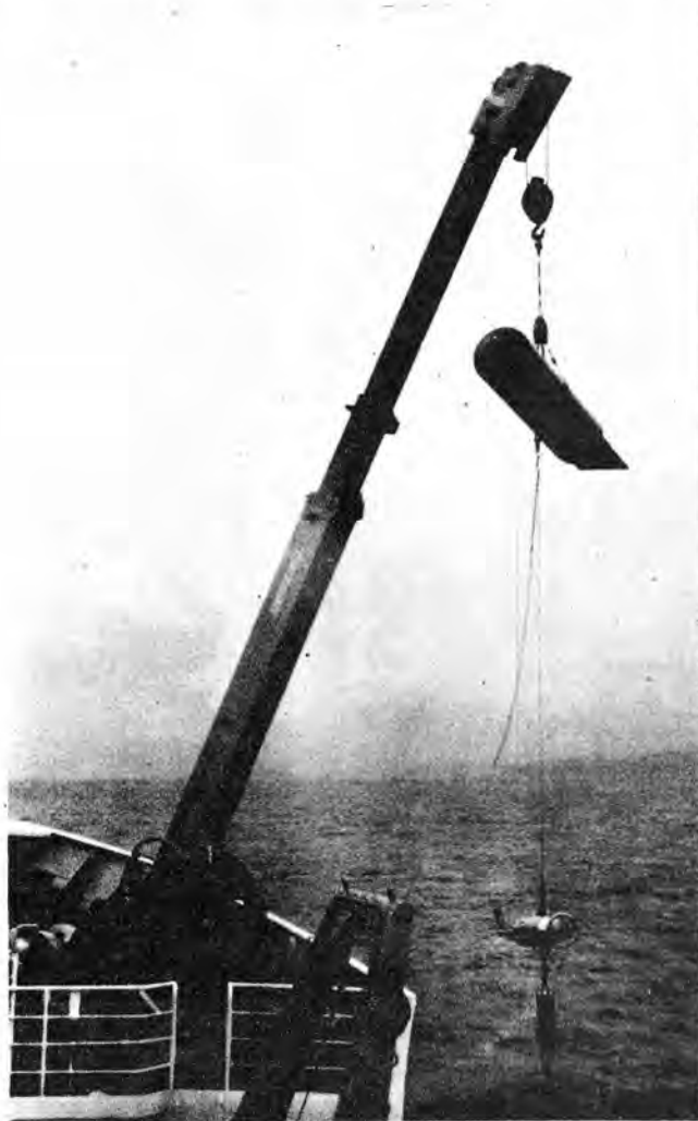
Figure 7 SUPPORT BUOY AND METER ON AUSTIN-WESTERN CRANE
